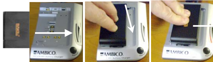
1) Insert the battery as shown 2) Push it down & hold 3) push to right to latch.
